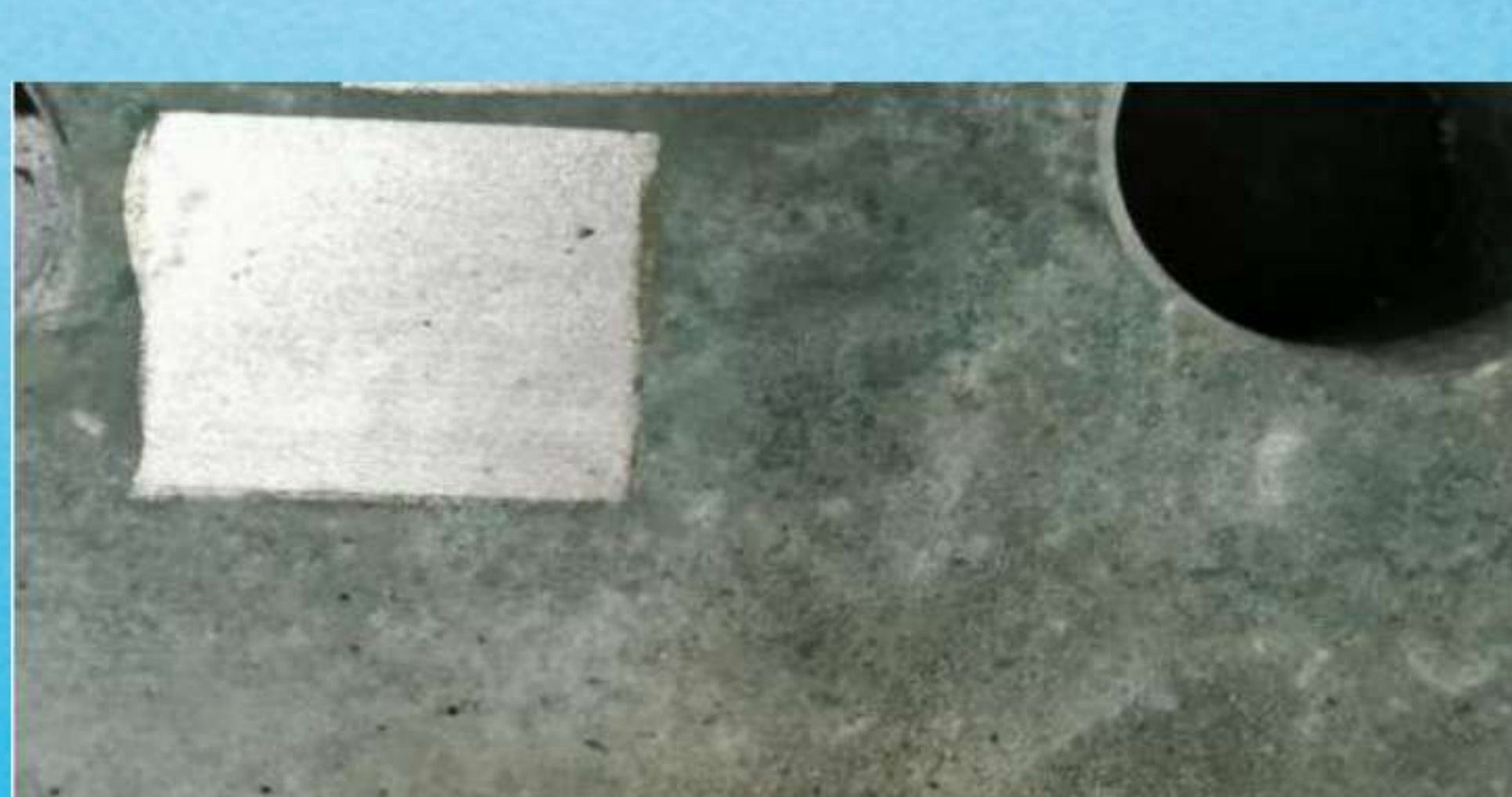
Copper alloy surface patina cleaning
